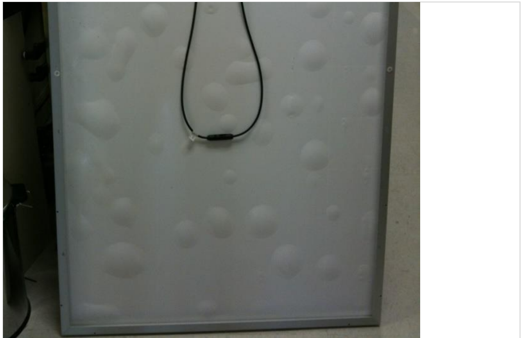
Figure 4.16 Module Failure Mode: Laminate Outgassing
