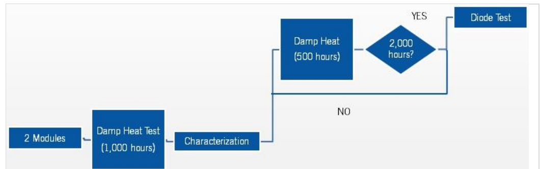
Figure 4.17 Damp Heat Test Procedure
