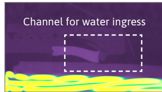
These XCT images show two poorly installed connectors. The top image reveals incomplete insertion and the left image zooms in on a channel for water ingress due to an undertorqued nut.
