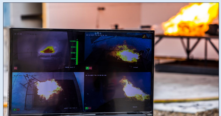
Fire testing (pictured above) reveals potential cell-level, module-level, unit-level and installation-level fire risks.
