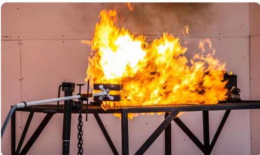
The image above shows a battery energy storage system in thermal runaway during destructive testing.
